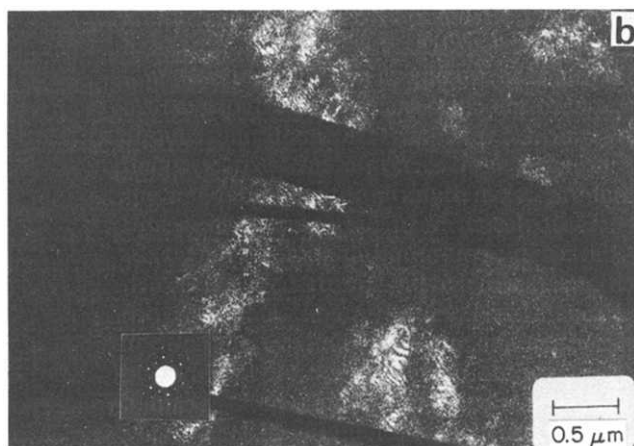
Figure 1(b) Dark field electron micrograph of a crystallized region (bright) and deformed regions (dark ribbons). Inserted is an electron diffraction pattern of the crystallized region
